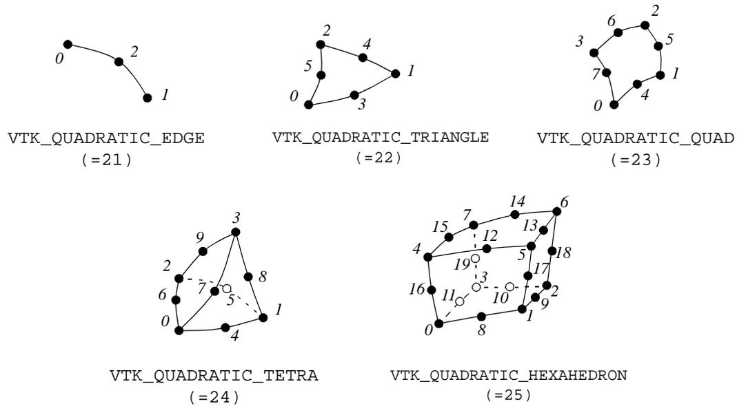
**Figure 3** Non-linear cell types found in VTK.
