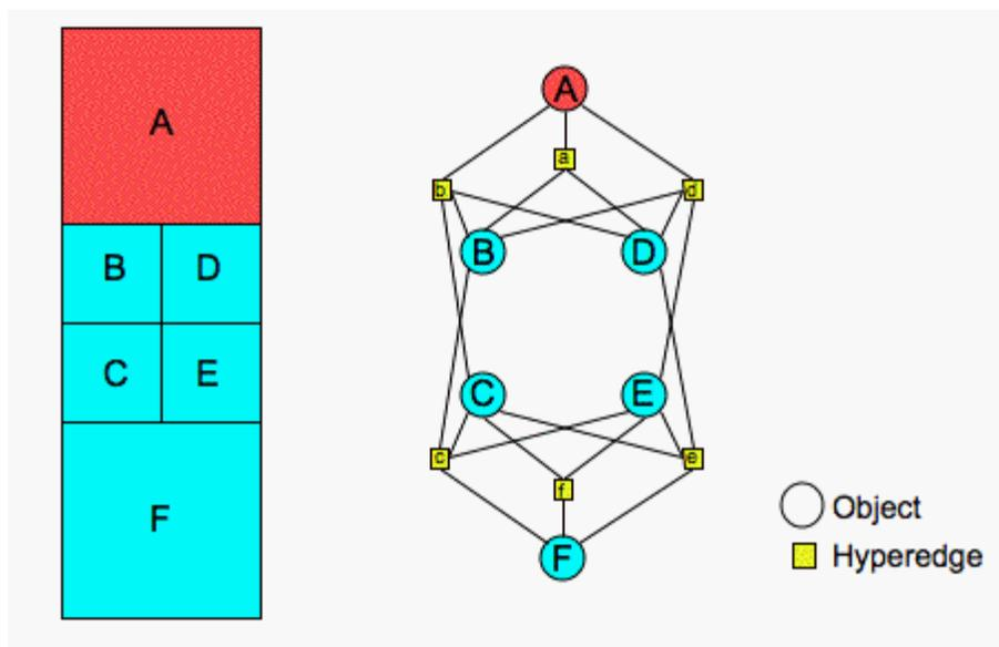
The blue and red shading indicates the mesh is partitioned for two processors. An application must provide information about the current mesh and partition to Zoltan. If, for example, the application wants Zoltan to perform operations on the elements of the mesh, it must provide information about the elements when Zoltan asks for object information.
